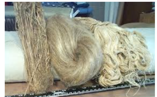
Above is an illustration of the dressed flax, from stalk fiber to yarn.
